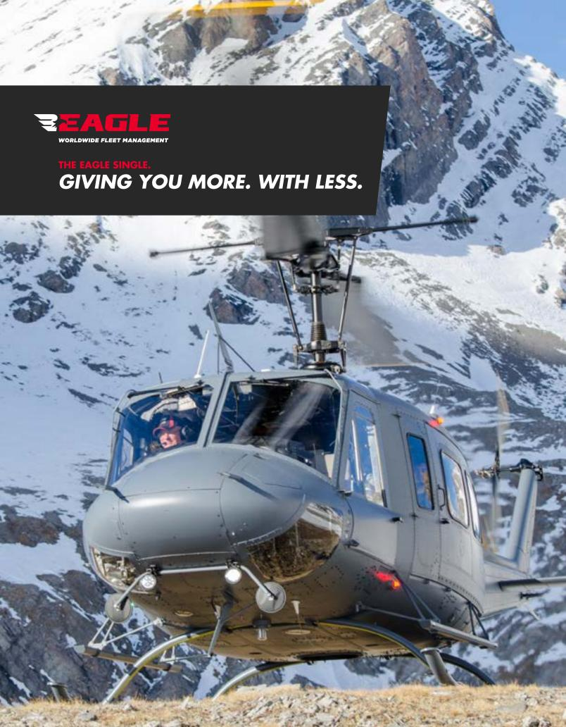
The EAGLE Single is the work horse in the Bell Medium Lift helicopter market. This program, by virtue of a 9-passenger Supplemental Type Certificate approval process, will convert the venerable Bell 212 helicopter from a twin engine to a single engine application.
